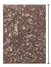
Structure -PTFE tape with proprietary filler system
