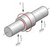
Fig. 10: Rotating load, shaft stationary, bush rotating
