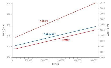
Fig. 3: Wear rate for GAR-FIL, GAR-MAX and HPMB
