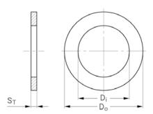
To order, specify MWXT size number plus suffix for desired thickness (062, 080, 125). e.g. MWXT1632-080 is a 1" ID x 2" OD x 0.080" thick GGB-MEGALIFE $^{\circ}$  XT thrust washer.
