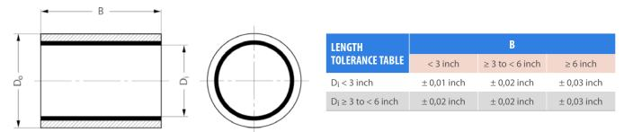
To order, specify bearing product prefix and size number plus suffix for desired length (in multiples of 1/16"). e.g. GM2428-032 is a 1.5" ID x 1.75" OD x 2" long GAR-MAX® bearing.
