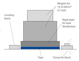
Fig. 5: Application of Multifil bearing tape
