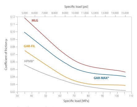
Fig. 4: Coefficient of friction vs specific load
