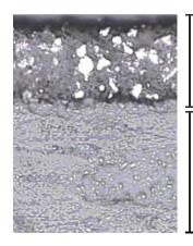
**Sliding layer** Continuous wound PTFE tape liner on both sides
