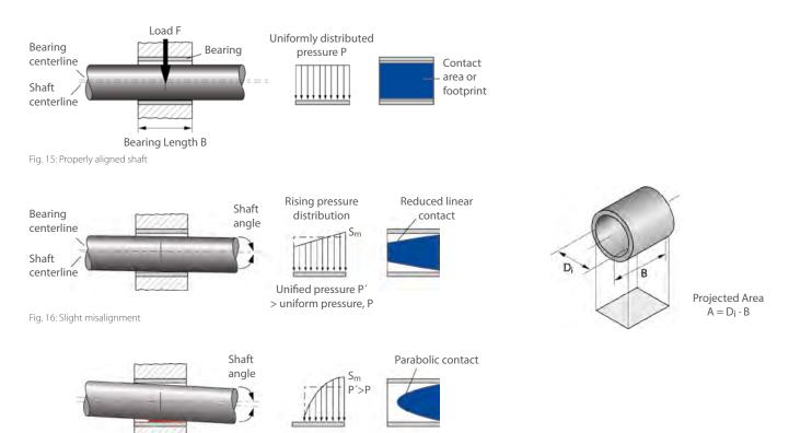
Fig. 17: Substantial misalignment
