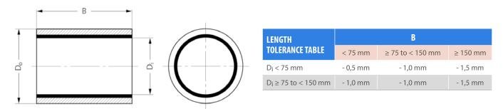
To order, specify bearing ID, OD and length size number (in millimeters) plus product suffix. e.g. 253020GM is a  $25 \text{ mm ID} \times 30 \text{ mm OD} \times 20 \text{ mm long GAR-MAX}^{\circ}$  bearing.
