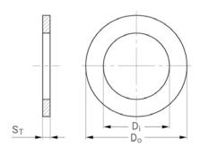
To order, specify MWXT size number plus suffix for desired thickness (15, 20, 30). e.g. MWXTM2244-20 is a 22 mm ID x 44 mm OD x 2 mm thick GGB-MEGALIFE® XT thrust washer.
