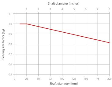
Fig. 13: Bearing size factor a<sub>B</sub>
