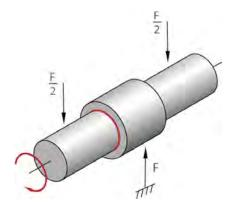
Fig. 9: Steady load, bush stationary, shaft rotating
