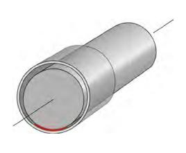
Fig. 14: Contact area between bearing and shaft
