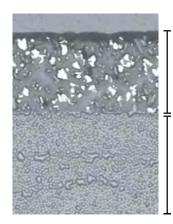
**Sliding layer** Proprietary filled PTFE tape liner
