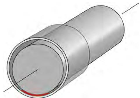
Fig. 14: Contact area between bearing and shaft
