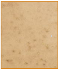
CuSn8 with Composition Sn 8 % P < 0,05 % Cu Rest
