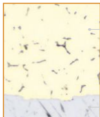
Sliding Layer CuSn8.5Bi7Zn2 Steel Backing
