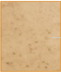
CuSn8 with Composition Sn 8 % P < 0,05 % Cu Rest
