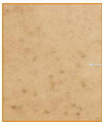
CuSn8 with Composition Sn 8 % P < 0,05 % Cu Rest
